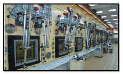
Hot cell facility at BARC for handling radioactive samples
